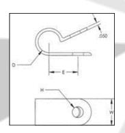
D: 6.35mm W: 12.70mm H: 5.16mm E: 10.41mm
