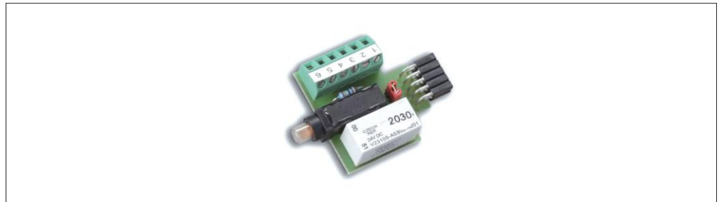
Fig.8-06 Optional signal and display control element SAB 04, front view
