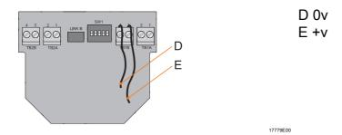
Reverse the polarity to activate the second sound tone frequency. The sounder PCB and beacon PCB must be wired independently if using reverse polarity to switch between sound tone frequencies.
