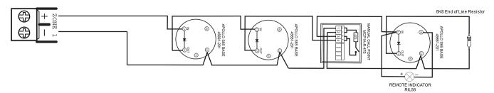
A maximum of 32 detectors per zone only can be fitted.
