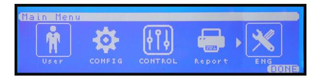
The Box surrounding the menu icon is the cursor, this is used to navigate through the menu options by using the Left/Right arrow keys to select required menu option and then press ✓ button.
