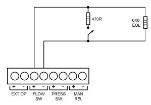
Figure Above: Typical Monitored Input Wiring
