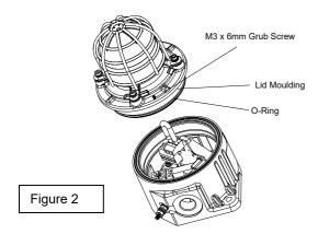
On completion of the installation the flameproof threaded joints should be inspected to ensure that they are clean and that they have not been damaged during installation.
