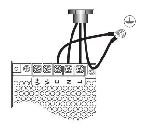
Sufficient earth lead should be left to allow Live and Neutral connections to be accidentally pulled from the terminal block while leaving the earth connection intact.
