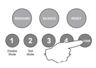
When finished, press and hold Button 1 (Disable Mode) for 3 seconds or alternatively wait approx 10 seconds and the panel will save the settings and revert back to Level 3 access mode.
