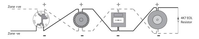
Haes Twin Wire systems require special 'sav-wire' detector bases and polarised call points but standard sounders. Most modern, non addressable, low current, polarised sounders, bells and beacons are compatible, Cooper Fulleon, Besson, Klaxon etc.
