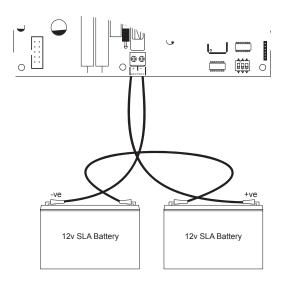
2 x 12v batteries should be connected in series using the white jumper lead provided. See diagram.
