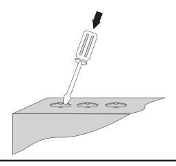
Knockouts should be removed with a sharp tap at the rim of the knockout using a flat 6mm broad bladed screwdriver.
