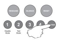
When finished all the zone function programming, enter the next programming code or disable the controls and return DIL switch 3 to 'OFF'.
