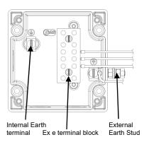
Note: Depending on options chosen an 8-Way DIN Rail or 6-Way terminal block may be selected.
