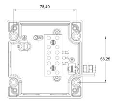
View of base unit showing fixing centres. To gain access to the mounting holes in the base the front cover must be removed. This is achieved by removing the 4 off M4 cap head bolts holding on the cover.
