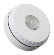
The Solista LX Ceiling visual alarm device (VAD) has a unique lens design that distributes the light in a cylindrical shape to achieve the required illumination specified by EN 54-23. Designed for installation at a height of up to 3m and with a discrete appearance, the device is ideal for a variety of applications, including bedrooms, bathrooms and toilets.
