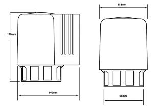
NOTE: The Master Blaster siren is only suitable for installations with a security or fire system control panel that provides a DC trigger signal.
