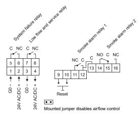
The relays are displayed in alarm mode, as they are in the event of a power outage.
